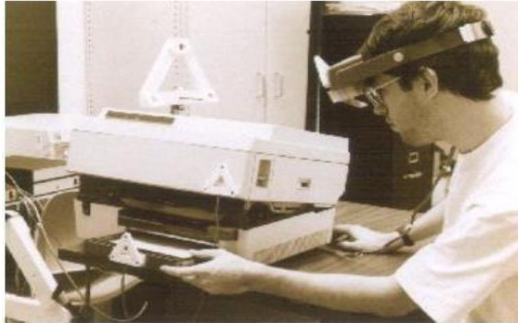
**Figure1: External view of Columbia printer maintain application. Noted that all objects are tracked.**
